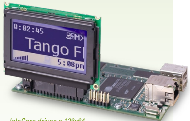
lalaCore drives a 128x64 graphics LCD module
