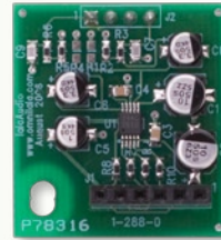
lala®Audio circuit – I2S to Analog module
